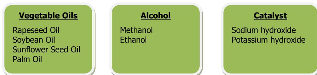
This section will describe the process of biodiesel production from vegetable oils where the triglyceride oil is broken into alkyl (biodiesel) and glycerine by reaction with a mono alcohol. The biodiesel and glycerine phases are then separated and purified. Production processes contain the same stages, irrespective of the production scale, although the differences in equipment may be significant.
